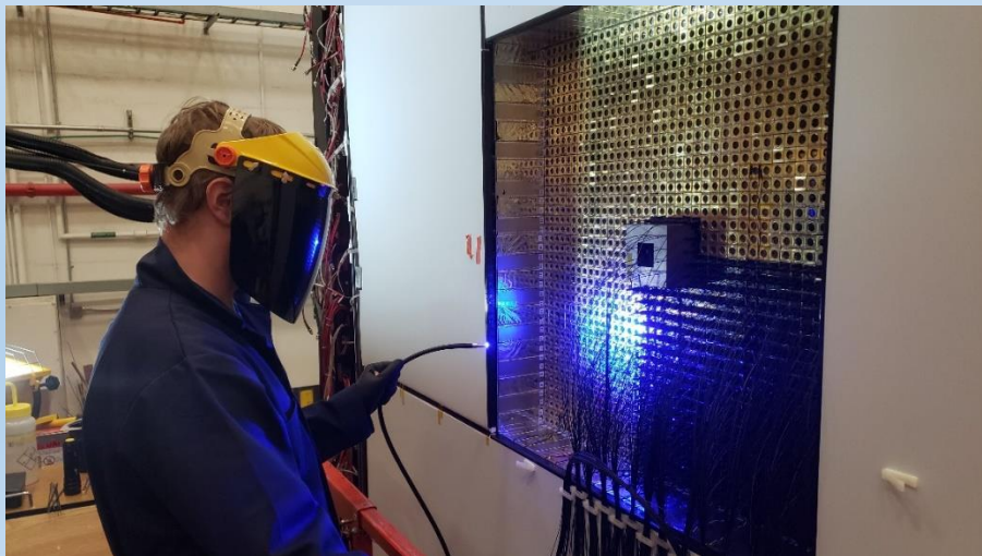
Gluing optical fibers to crystals (UV curing)
