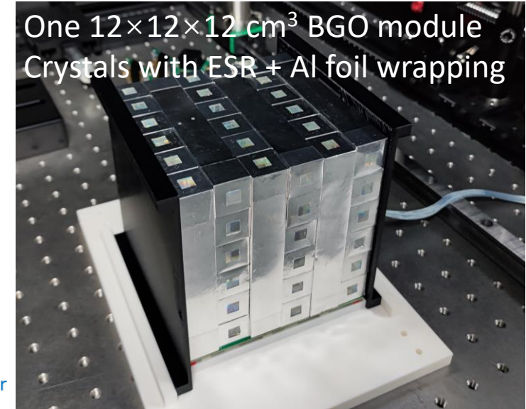
Support structure design and module assembly test
