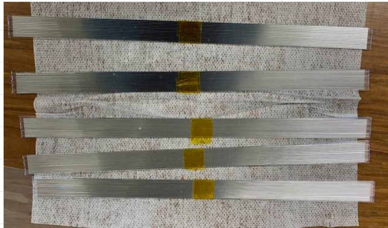
1mm sq Scin. Fiber (14) and 0.15mm W-strip
