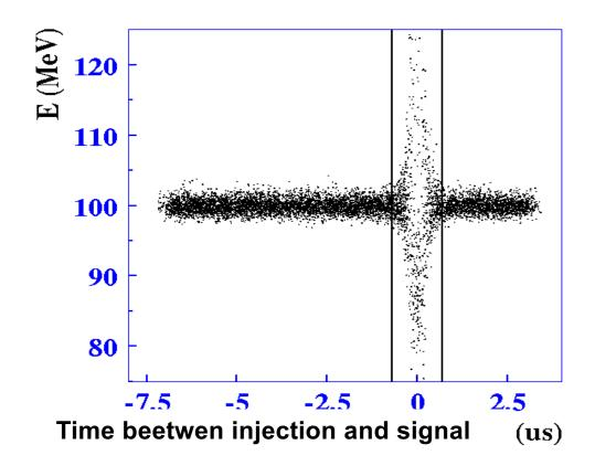
The time cut can be reduced to  $\pm$  0.6 mks without resolution degradation
