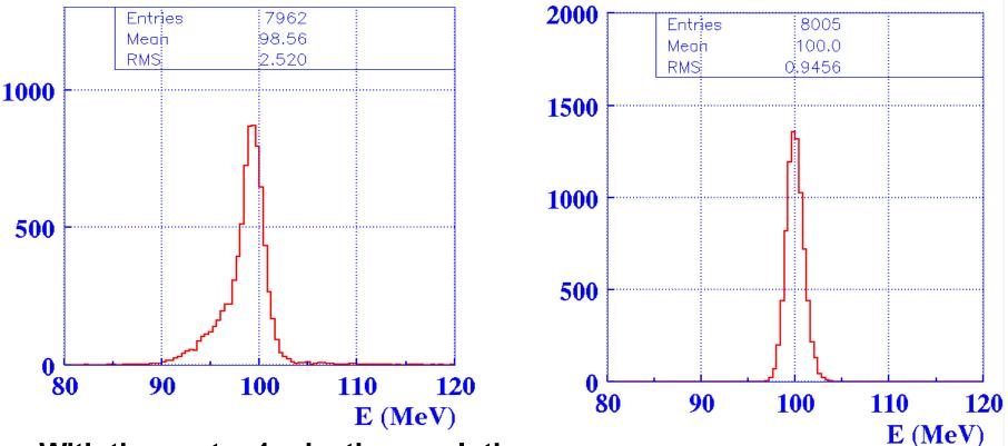
With time cut +-1 mks the resolution and peak position are the same as without injection
