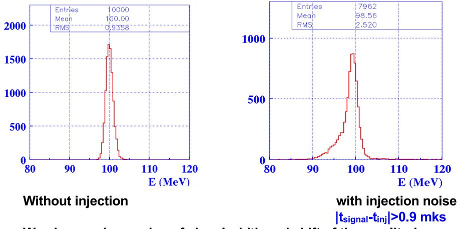
We observe increasing of signal width and shift of the amplitude
