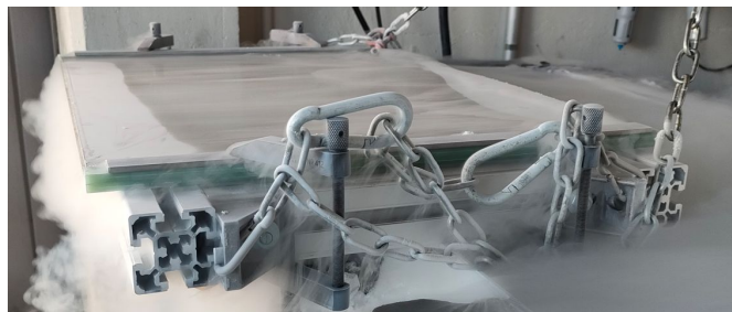
Test beam prototype. 64 electrodes and absorbers.
