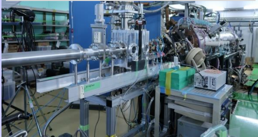
The 7 MeV proton accelerator
