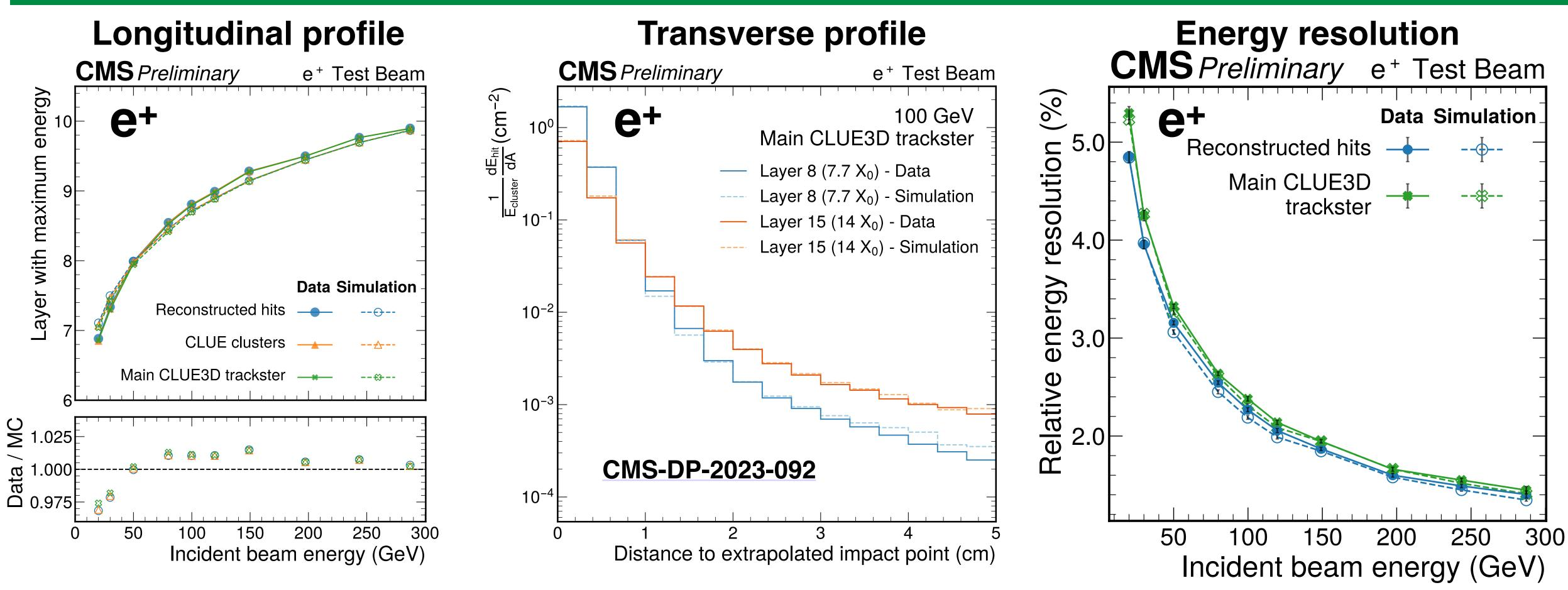
Performance of CLUE and CLUE3D in test beam data well described by simulation.
