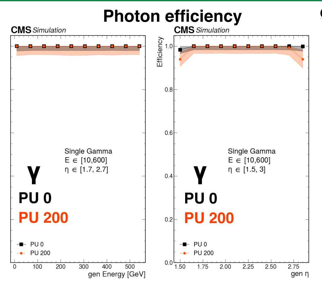
Reconstruction of electromagnetic objects show high performance up to 200 PU.
