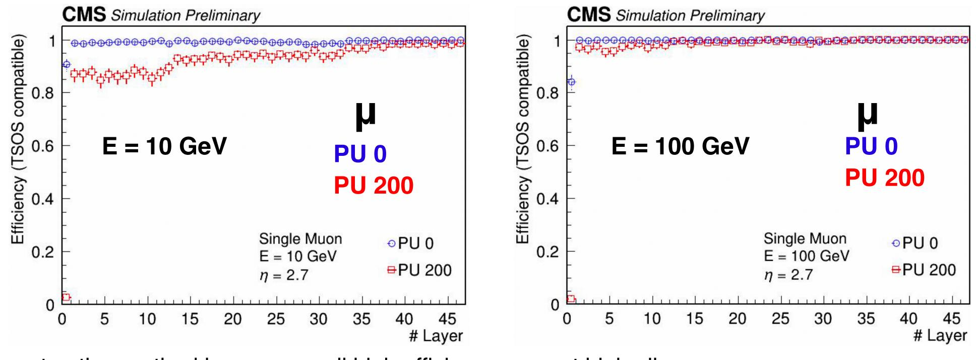
Muon reconstruction method has an overall high efficiency even at high pileup.
