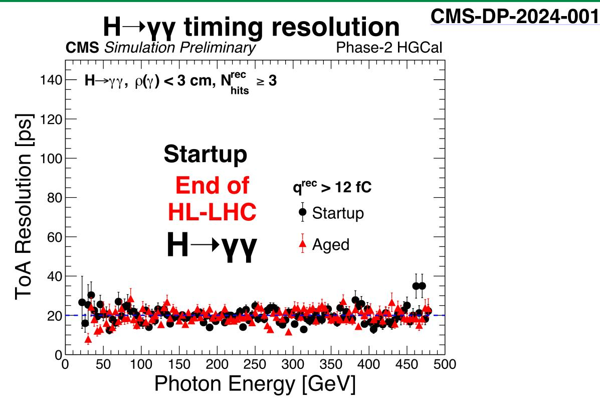
• High efficiency for time tagging neutral hadron showers at E > 20 GeV, maintaining a timing resolution ~ 20 ps
