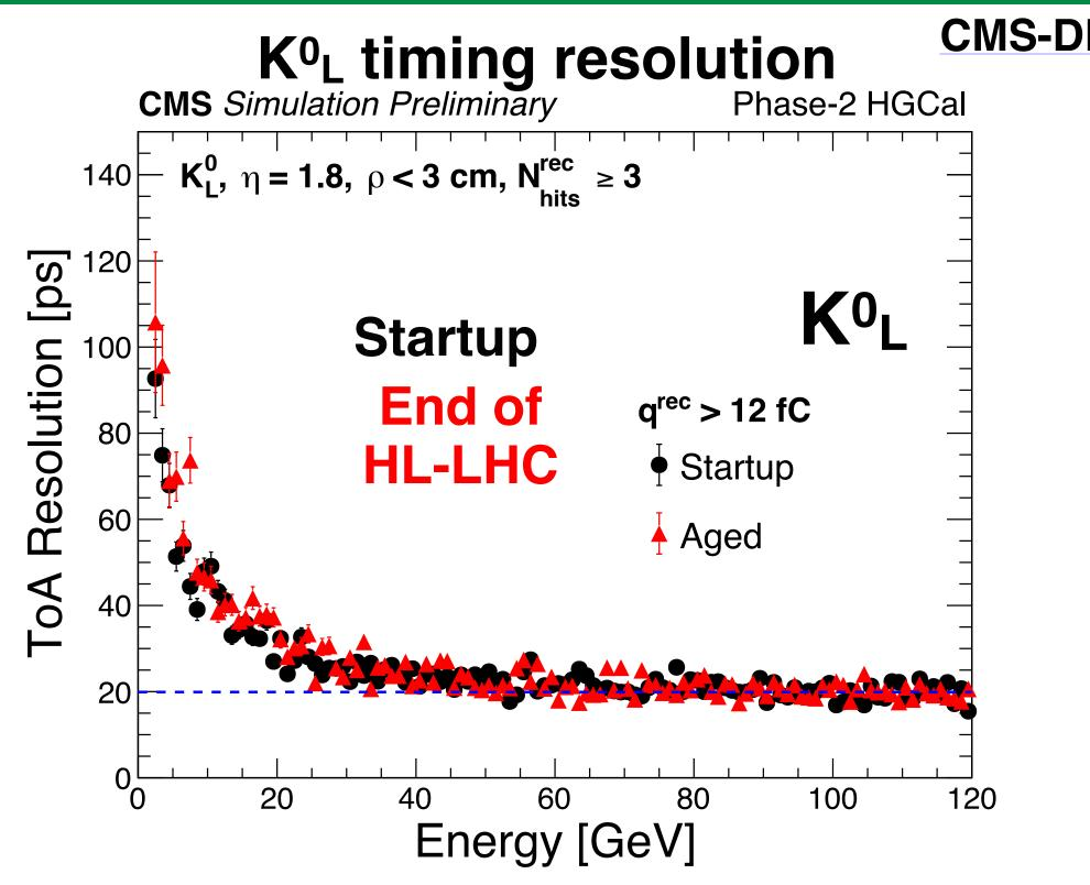
• High efficiency for time tagging neutral hadron showers at E > 20 GeV, maintaining a timing resolution ~ 20 ps
