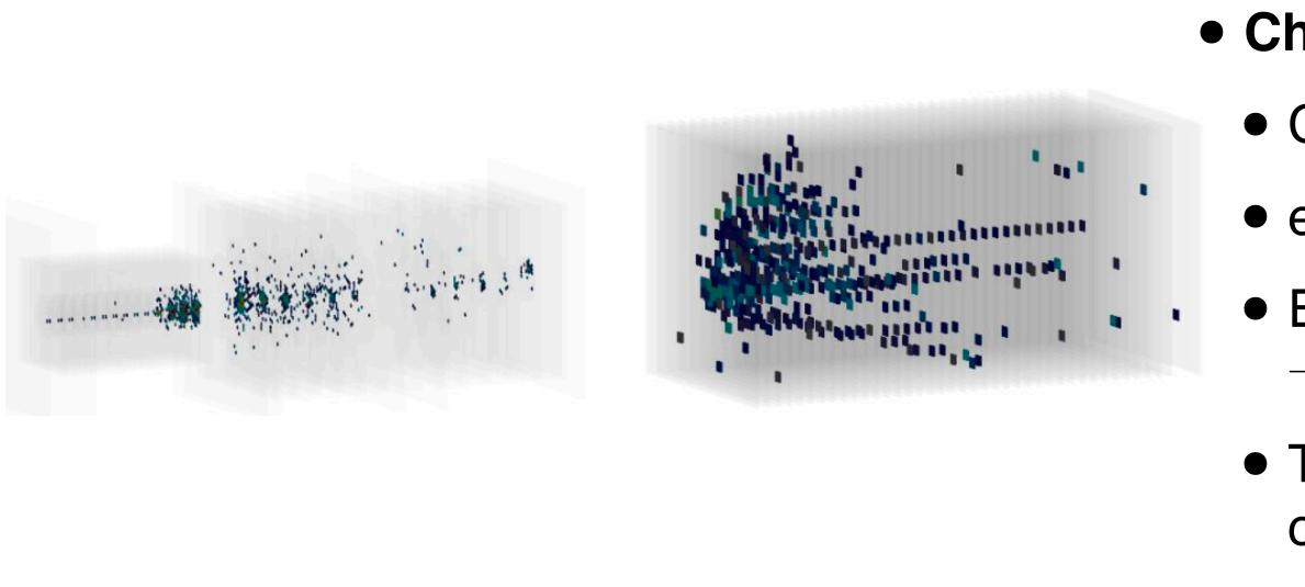
• Dynamic graph neural networks (GNN) models can be used to tackle these challenges and fully exploit the HGCAL granularity by connecting rechits using their energy and spatial information through graph convolutions.
