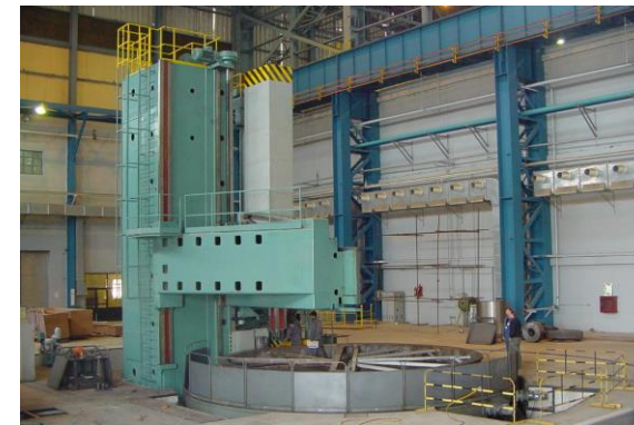
16m vertical boring and turn mill (3-axis CNC) at PAEC in Pakistan
