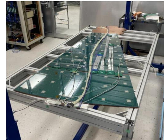
20° mixed cassette mechanical mockup
