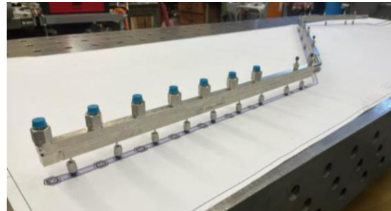
On-detector manifold optimisation: reduced number of welds (KIT proposal)
