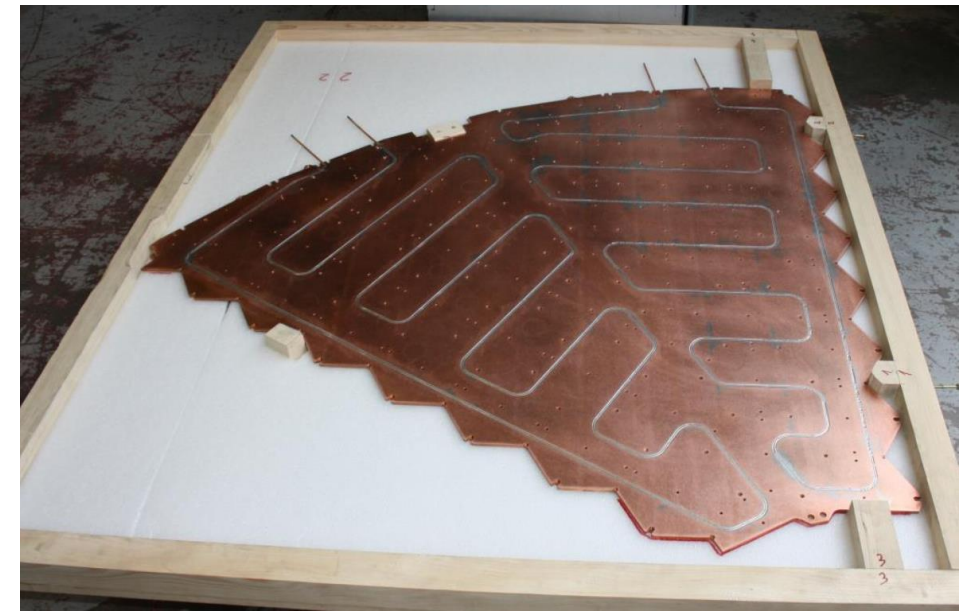
CE-E copper plate prototype with embedded cooling pipe
