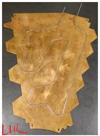
Pipe insertion on a cooling prototype
