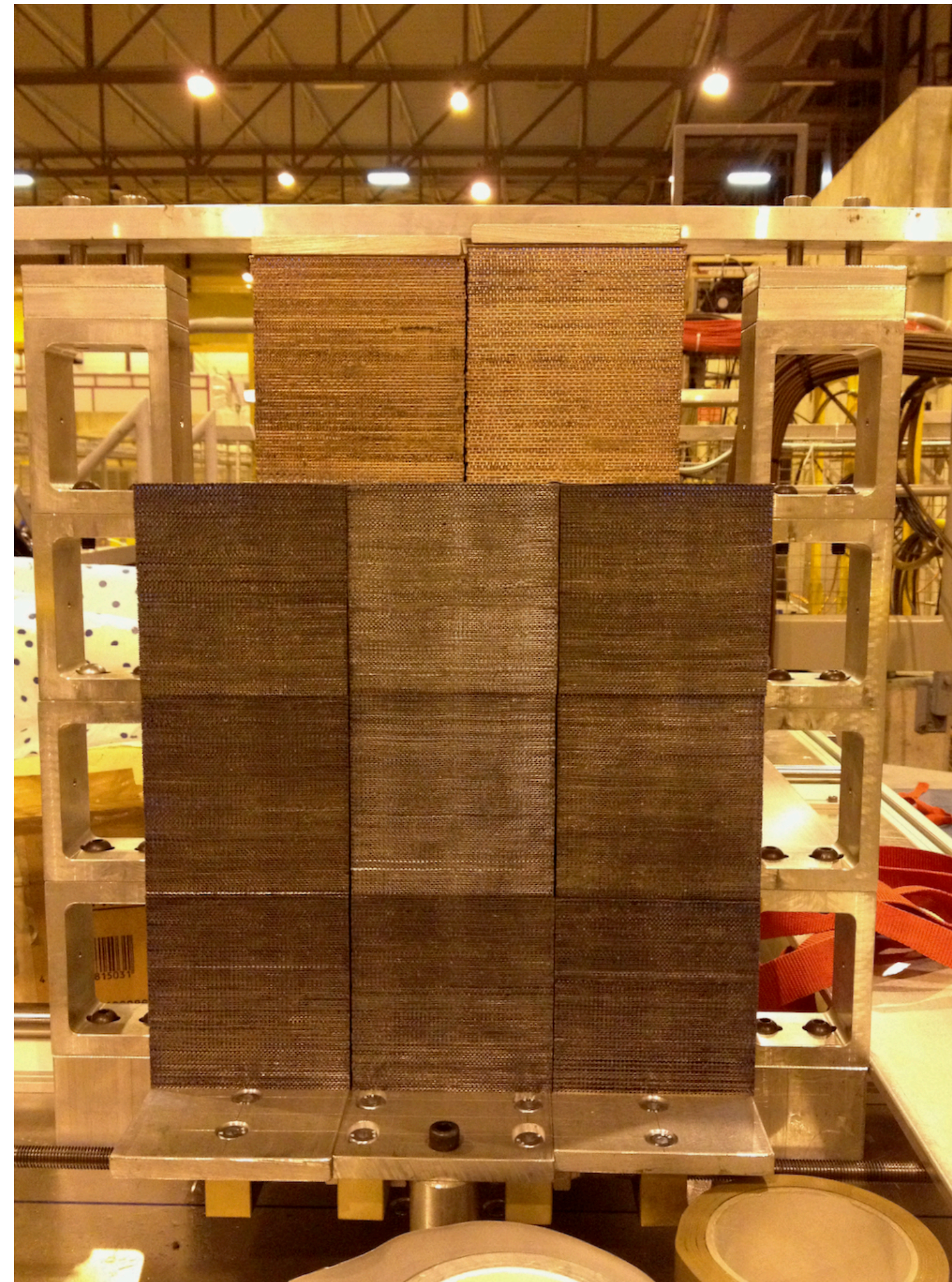
Fig. 2. Pictures of the first SuperDREAM modules built with lead (left) or copper (right) as absorber material. The alternating arrangement of clear and scintillating fibers in each row of the copper modules is illustrated by illuminating the fiber bunches from the rear end.
