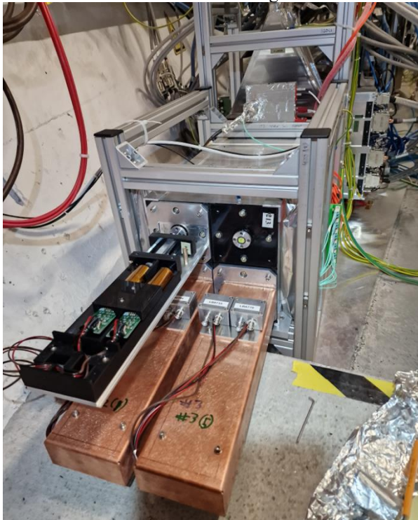
Fig. 8. Upgraded PMT system during installation.
