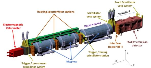
**Figure 1.** A sketch of the FASER detector, showing the different sub-detector system. The detector coordinate is also shown [2].
