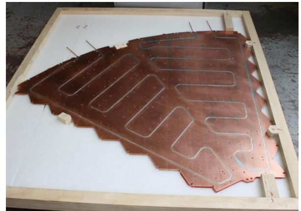
Fig. 6. CE-E copper cooling plate prototype
