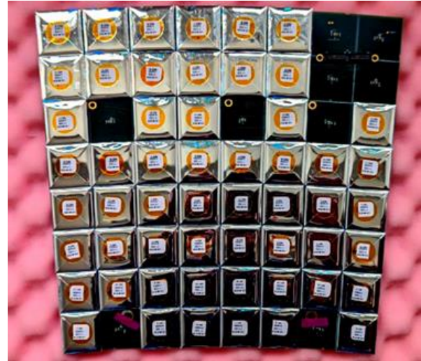
Fig. 3. Tileboard with wrapped tiles on top of SiPMs
