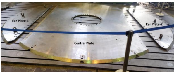
Fig. 5. CE-H absorber disc in three parts
