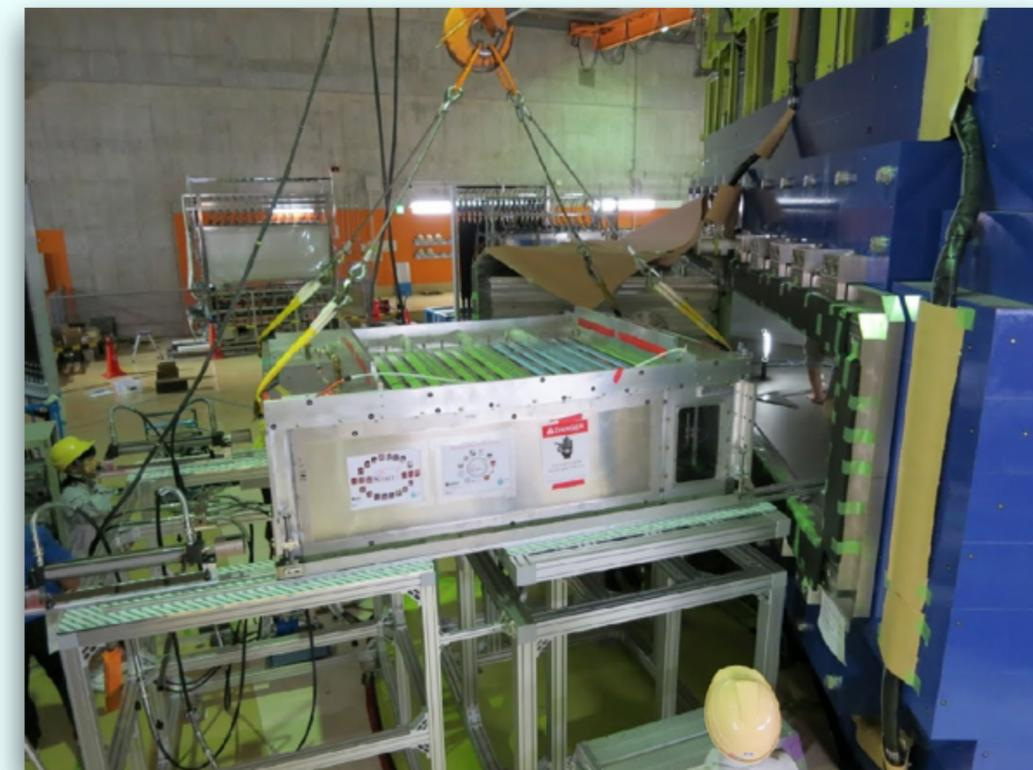
$S\pi$ RIT-TPC was installed inside the SAMURAI dipole magnet.
