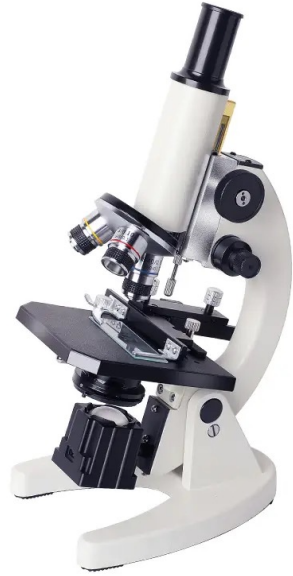
Optical microscope Photon \rightarrow Target material Observation scale: 10^{-7} m
