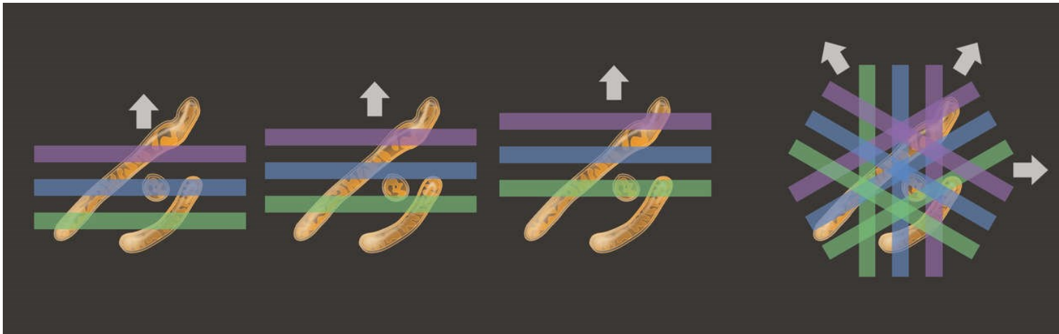
Figure 9 [14] – Capture multiple images with structured illumination that is shifted in phase. Repeat this process for three different angles. These images are then processed using advanced algorithms to obtain super-resolution images.
