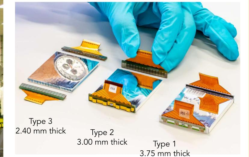
Upgrades needed: a new timing layer will be installed into CMS to mitigate PU. The MIP Timing **Detector** (MTD) will provide time resolution of 30-60 ps
