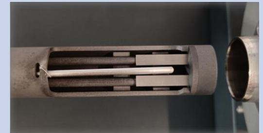
View on in-plane samples installed in graphite sample holder
