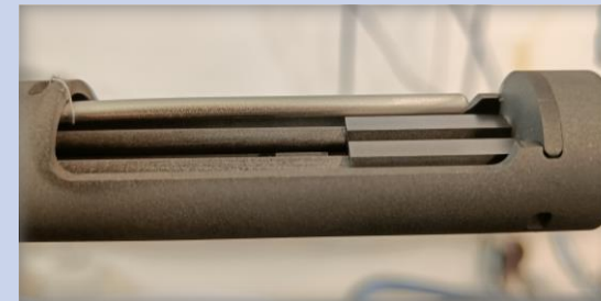
View on in-plane samples installed in graphite sample holder
