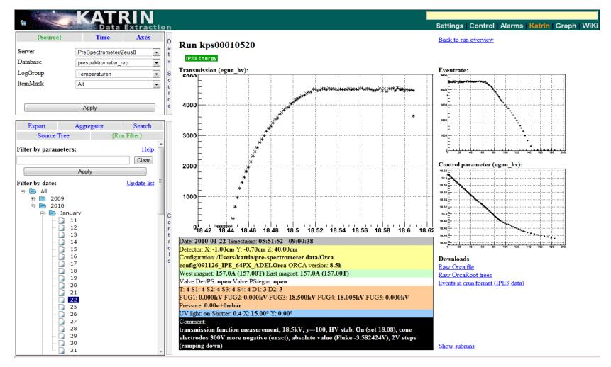
Combined SlowControl and DAQ data: Pixel detector hit rate over electron gun voltage.
