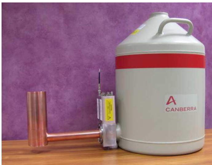
CDEX-1B (1kg PPCGe), cooled with the cooling finger and LN2 Dewar
