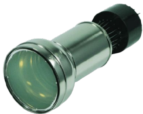
Geometry of the PMT matrix (left) and photo of Hamamatsu R11410-20 (right)
