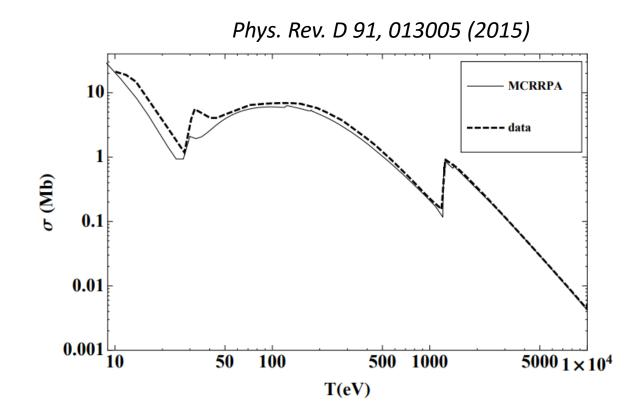
The photoabsoprion cross section reflects the atomic shell structure.
