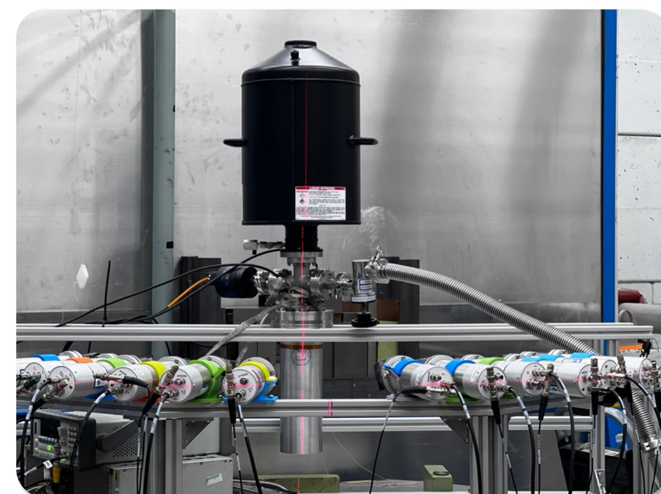
Fig. 4: Setup for 77 K QF measurement at TUNL.
