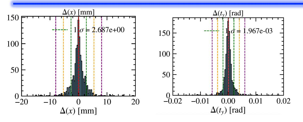
Hits in Pixel-Fibres matched, fitted and extrapolated back to VELO exit. Then the track state parameters are compared with the truth values.
