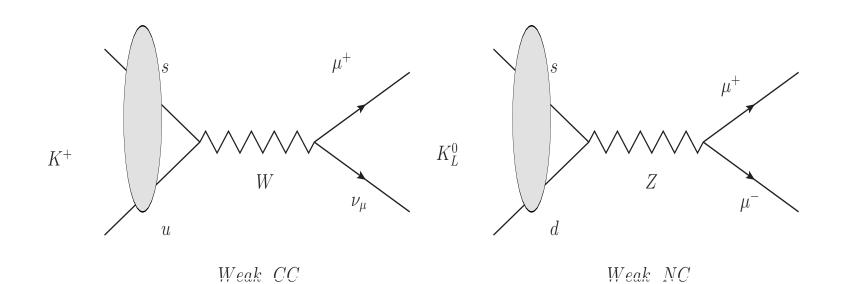
$K^+$ ,  $\bar{s}u$  bound state.  $K^+ \rightarrow \mu^+ \nu_{\mu}$ : weak charged current decay,  $\Delta S = 1$
