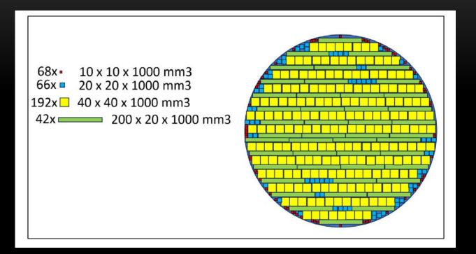
The shielding design recently approved by the Machine Group has 1m of iron arranged in the Duct as shown and supersedes our original proposal of 2m of concrete
