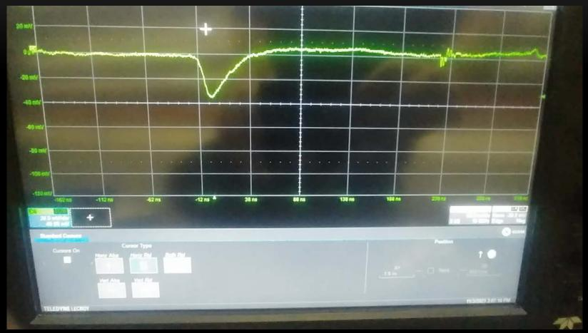
Each installed PM is checked using cosmic rays that still manage to penetrate the 105m overburden
