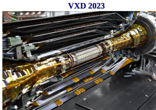
• SVD and fully-equipped PXD mounted around modified beam pipe (Au coating, cooling)
