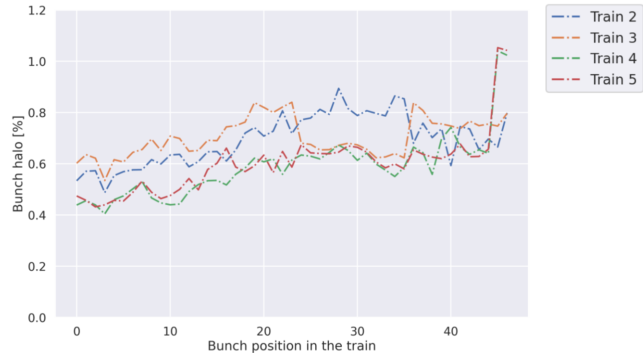
Figure – Bunch-by-bunch halo left in B2H and right in B2V.
