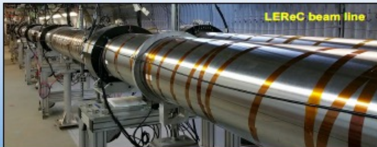
LReC: First-ever electron cooling with bunched beams Test case for electron cooling at EIC
