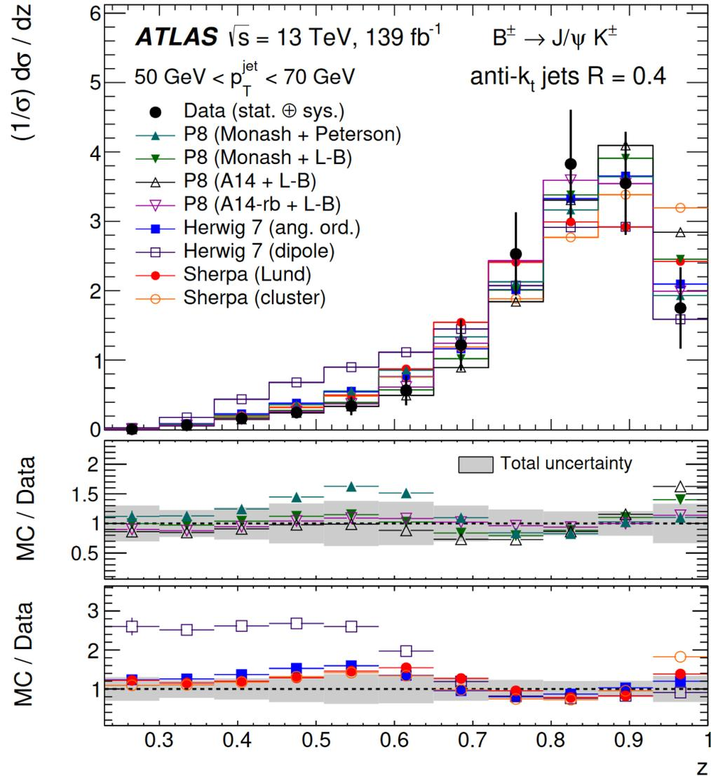
$$z = \frac{\vec{p}_{\text{jet}} \cdot \vec{p}_B}{|\vec{p}_{\text{jet}}|^2}$$
