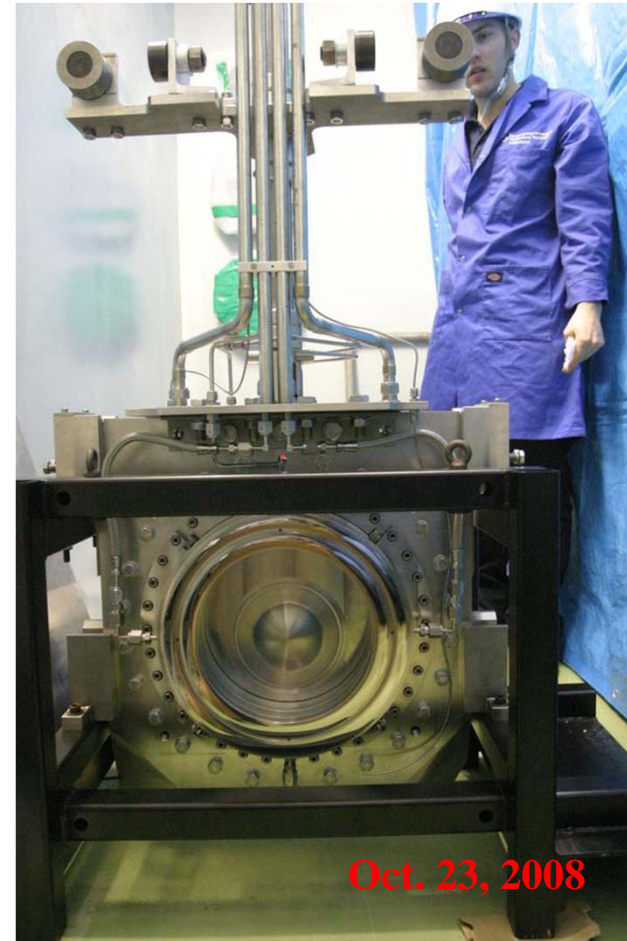
The Ti-alloy beam window cooled by He gas
