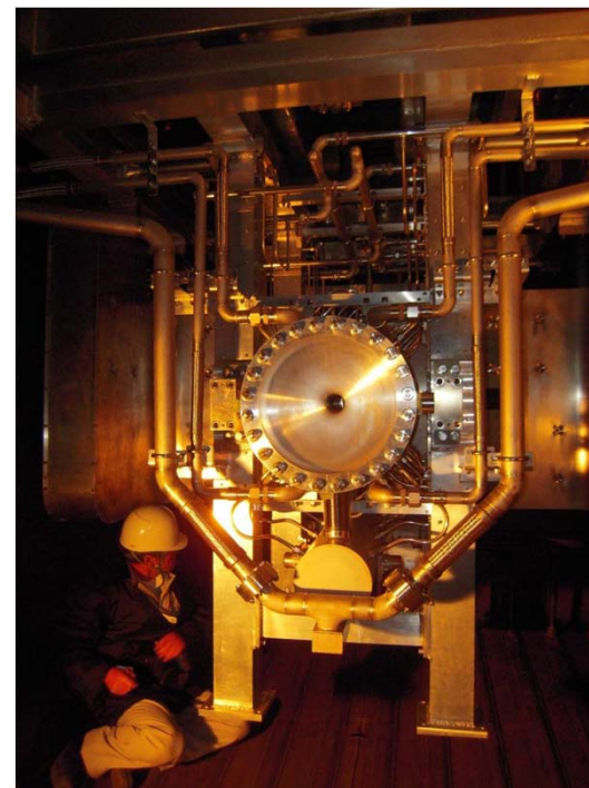
Target: 26mm- \phi x 900mm-L graphite
