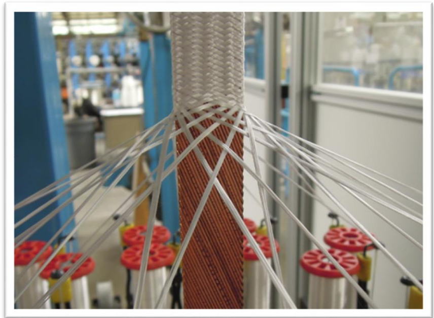
Fiber glass insulation for Nb 3 Sn
