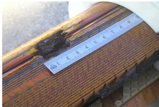
Result of degradation due to local heating in a NbTi coil
