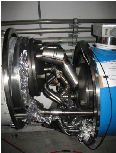
Result of the chain of events triggered by a quench in an LHC bus-bar
