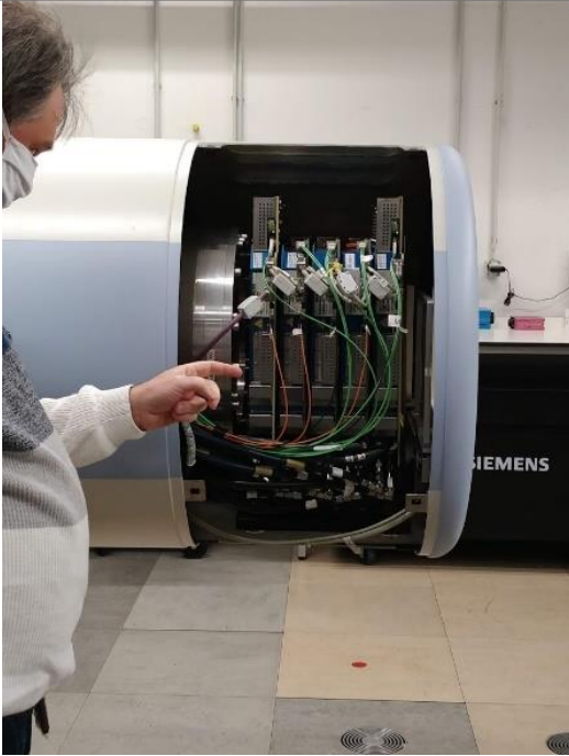
One beam nozzle. It's at end of the beamline, with BAMS inside the nozzle.
