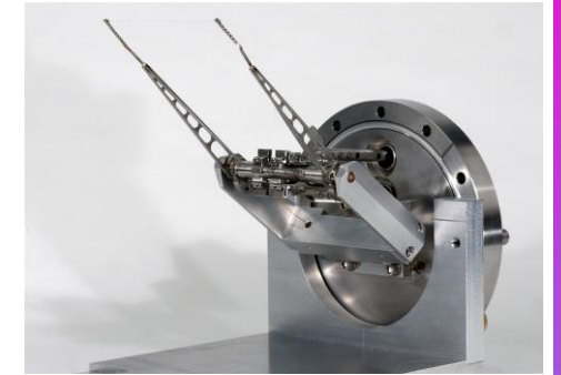
Beam wire scanners
