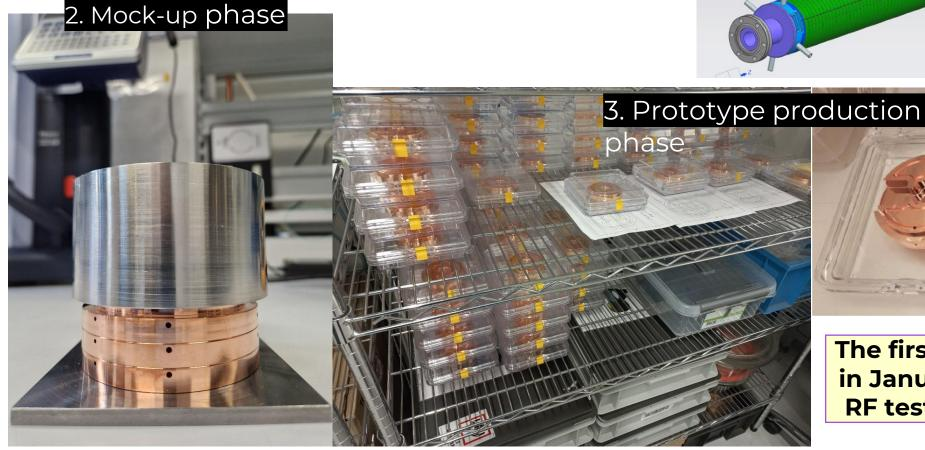
The first structure will be brazed in January 2024 with low power RF tests beginning of February 2024.
