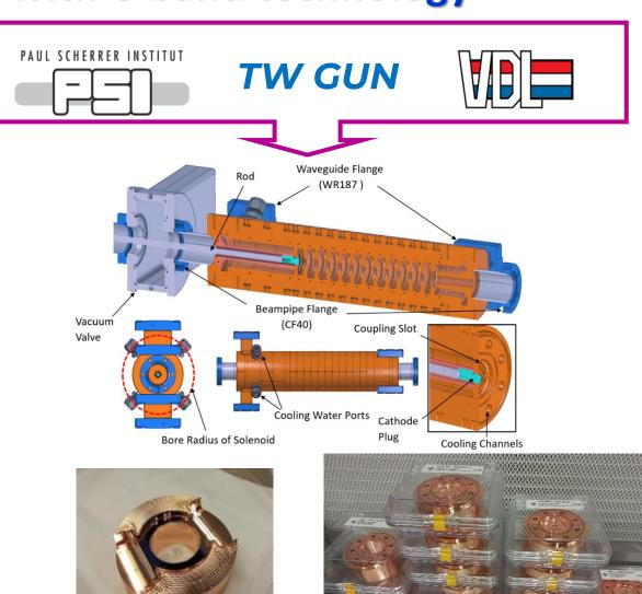
Travelling Wave gun design completed: cells and couplers under construction at VDL (expected final
