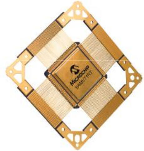
Microchip microcontroller using 150nm technology node
