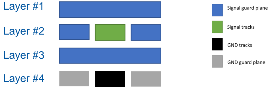
Schematic of the cross section of the test board showing the 4 layers
