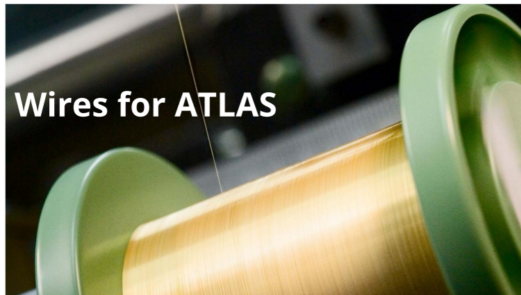
Luma Metall Luma Metall in Kalmar has developed into a specialist in the plating of fine and ultrafine wire in tungsten and molybdenum, two materials traditionally used for filaments in light bulbs. From being Sweden's most well-known brand of incandescent lamps, Luma is now a high-tech supplier of fine wire products and precious metal plating technologies to research facilities and industry. In 2019 Luma received a significant order from CERN for more than 400 km of wire, to be used in the upgrade of a detector in the Atlas experiment at CERN. The material that Luma is supplying consists of 50-micron (= 0.05 mm) base tungsten wire on which a gold plating is added (about 0.35-micron pure gold).
