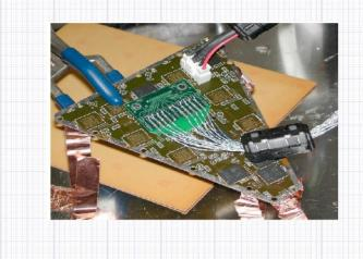
Lund – Transition Radiation Tracker: • Tension plates for barrel TRT • Front-end electronics cards • Digital integrated read-out circuit, DTMROC
