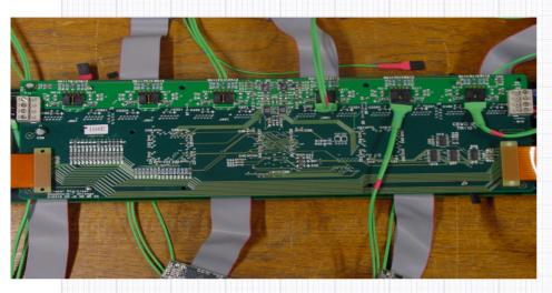
Stockholm – Tile Calorimeter: Production of front-end readout electronics
