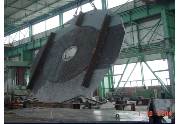
Test assembly of JD disks at the “Lola factory” in October 2004
