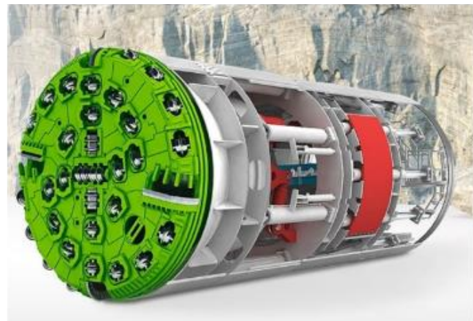
Tunnel Boring Machine (TBM)
