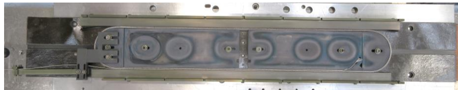
Measurement of coil length at CEA
