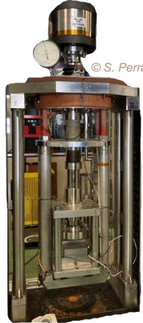
Cryostat & machine for 10-stack test
