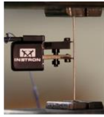
Nb_3Sn strand w/ extensometer for tensile test
