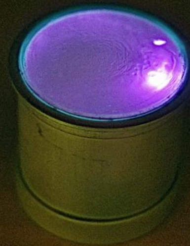
NaI (Sodium Iodide) detector for \gamma radiation
