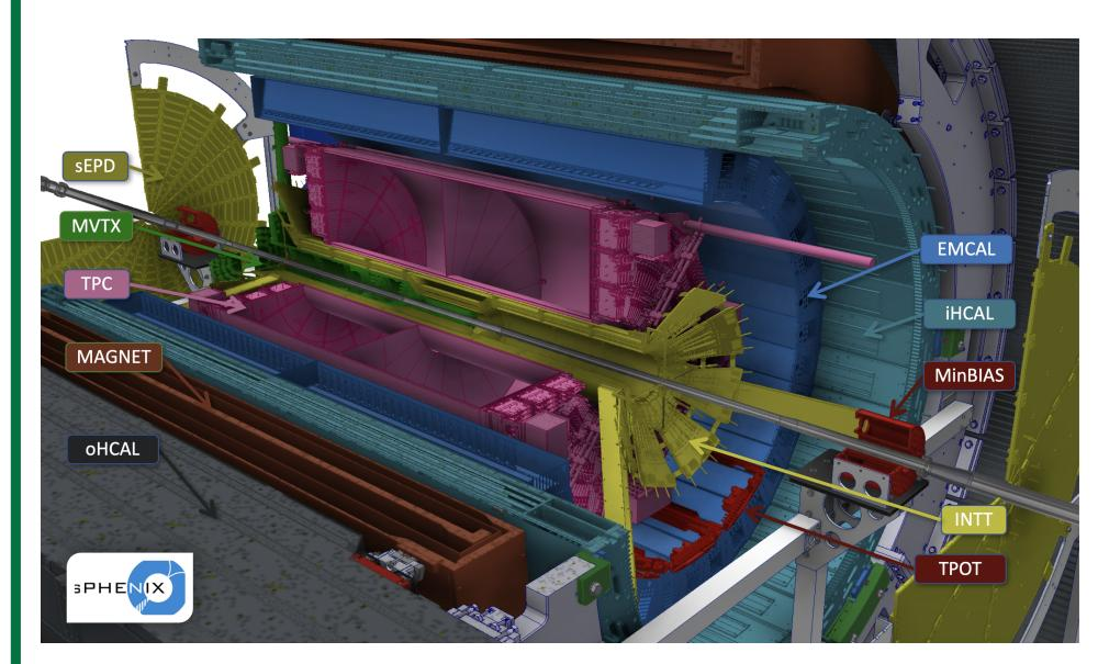
Multiplier (GEM) foils are Gas Electron quad-stacked, modules 36 are placed per side. contains Each stack  $\operatorname{two}$ pitch planes. standard large and  $\operatorname{two}$
