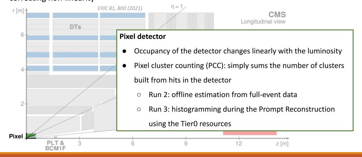
Requirement: linear signal-luminosity dependency or measuring and
