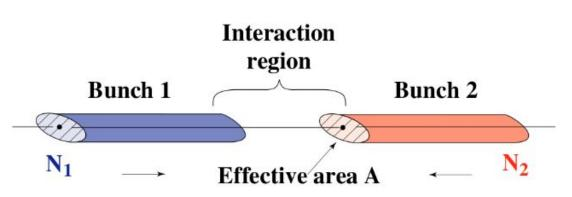
$$\mathcal{L}_{inst}^{i} = N_{1}^{i} N_{2}^{i} f \int \rho_{1}(x, y) \rho_{2}(x, y) dx dy = N_{1}^{i} N_{2}^{i} f \int \rho_{x1}(x) \rho_{x2}(x) dx \int \rho_{y1}(y) \rho_{y2}(y) dy$$
