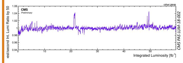
long-term comparison of the measured luminosities by various independently calibrated luminometers
