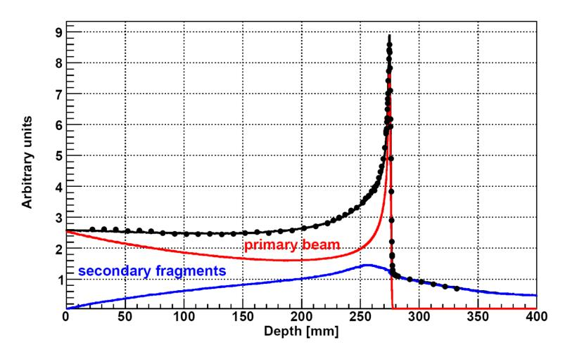
Bragg peak in a water phantom 400 MeV/A C beam:
