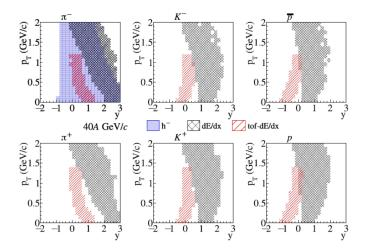
The final spectra of identified primary particles is corrected for detector geometrical acceptance and reconstruction efficiency as well as weak decays and secondary interactions.
