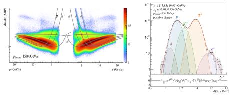
dE/dx analysis uses energy loss information of charged  $\pi$ , K, p in TPCs to identify particles. The curves calculated using the Bethe-Bloch function show the expected dependence of the mean dE/dx on momentum for the particle.
