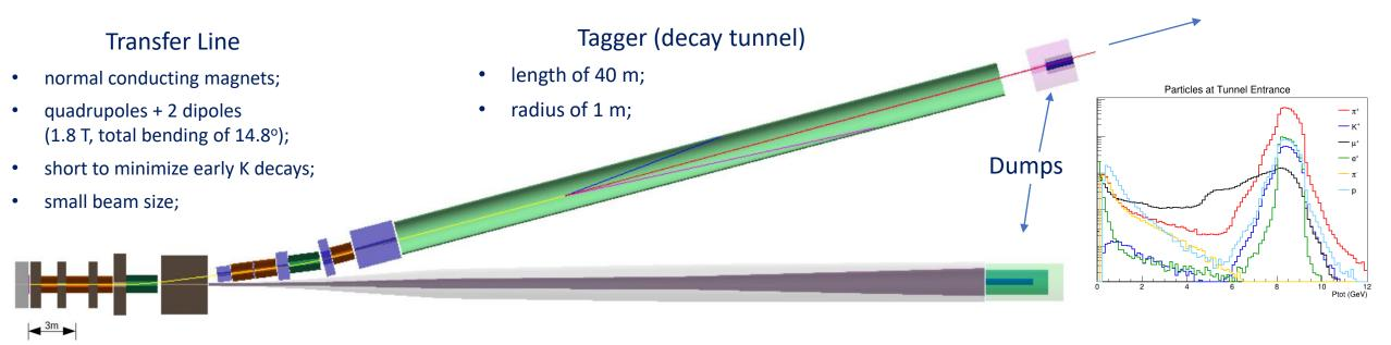
Large bending angle of 14.8°: better collimated beam + reduced muons background + reduced  $v_e$  from early decays;
