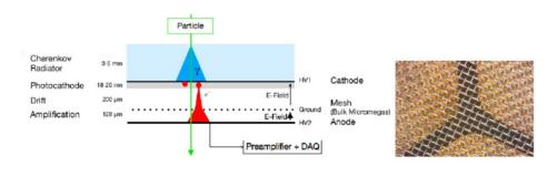
Possible candidates: fast Micromega detectors with Cherenkov radiators (PIMENT)
